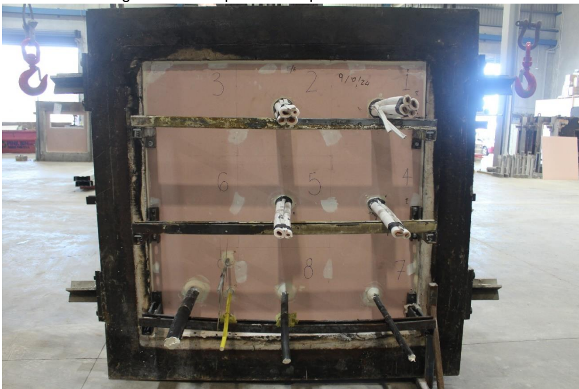
Figure 2 – Exposed face prior to test commencement
